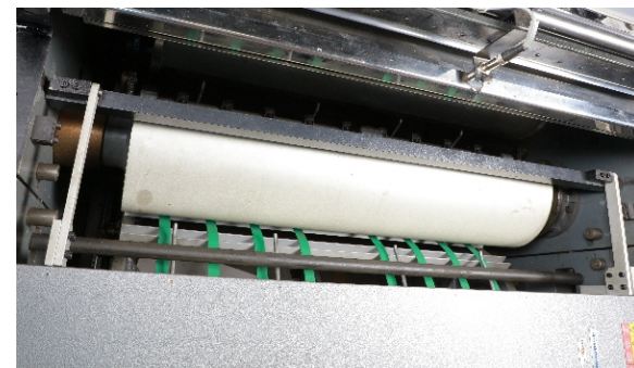
Transfer Cylinders with Anti-Marking Glass Bead Sheets The Transfer Cylinders are covered with Anti-Marking Glass Bead sheets which ensures the coated sheets are transferred smoothly without any scratches or marks.
